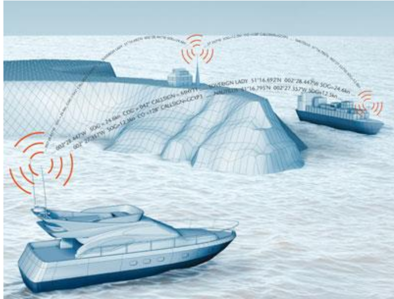
Figure 5: Visual Representation of data transfer through VHF. Source: IMO
